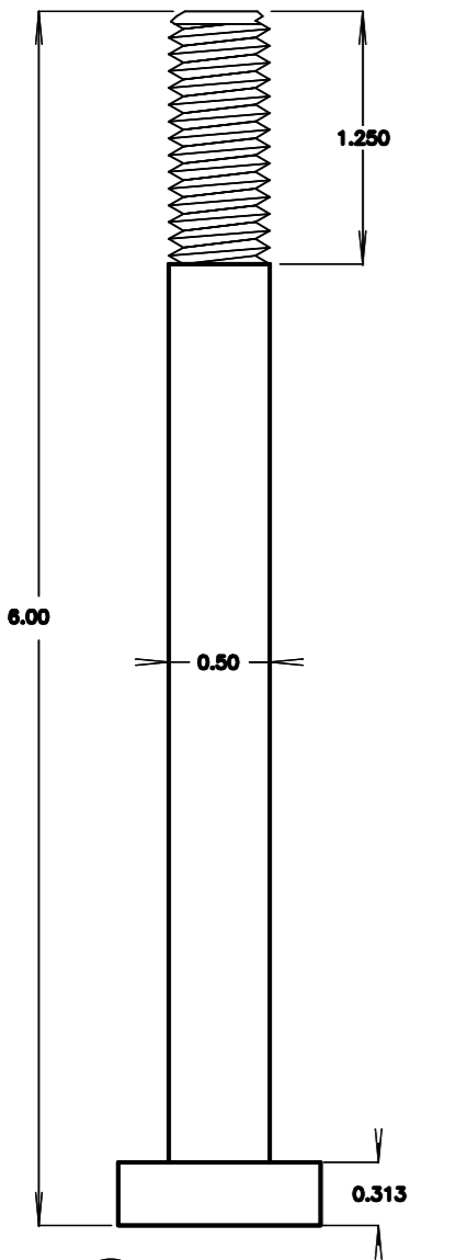
4 BOLT MAT'L SAE 1040 HEAT TREAT 1 REQ'D
